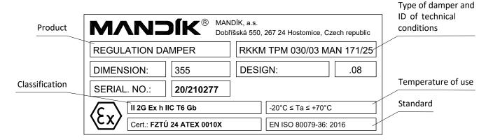
In the case of a damper equipped with an actuator, the assembly is additionally marked with an assembly label containing:
